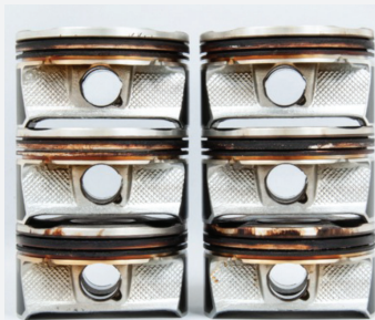
Figure 1: Front engine piston appearances after 90h of testing per Sequence IIH (ASTM D8111).
