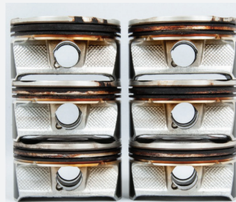
Figure 2: Rear engine piston appearances after 90h of testing per Sequence IIH (ASTM D8111).
